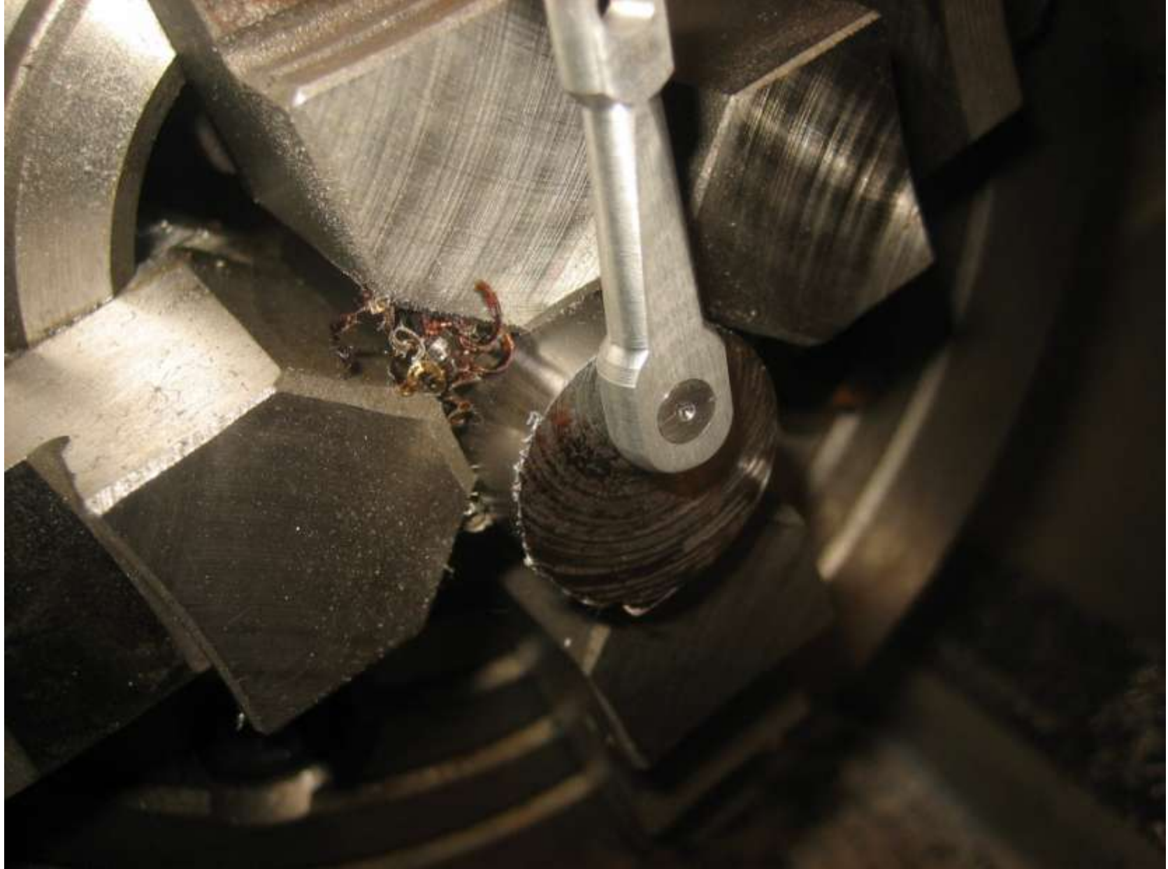
Testing the conrod before removing
