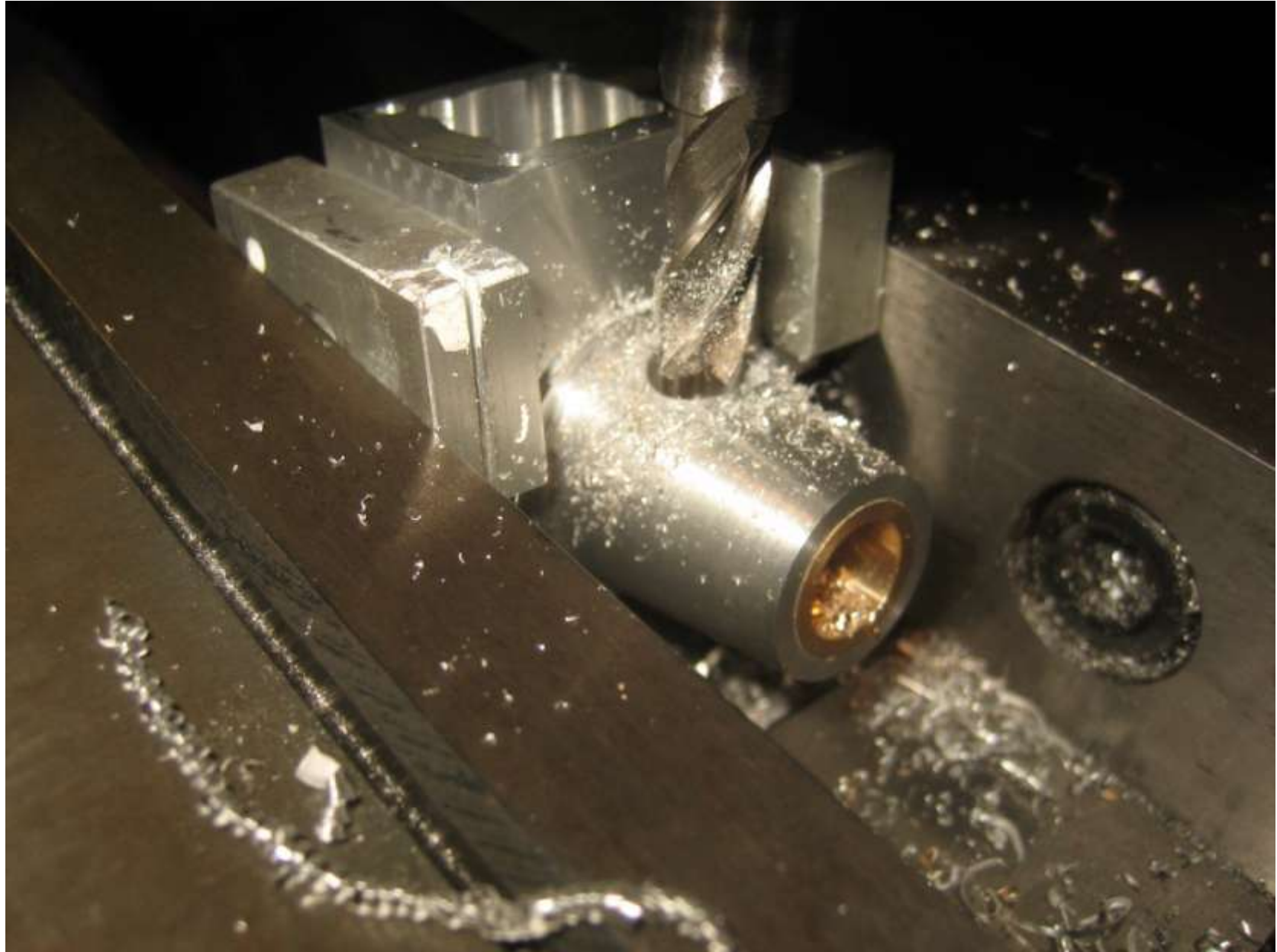
Machining the venturi hole.
