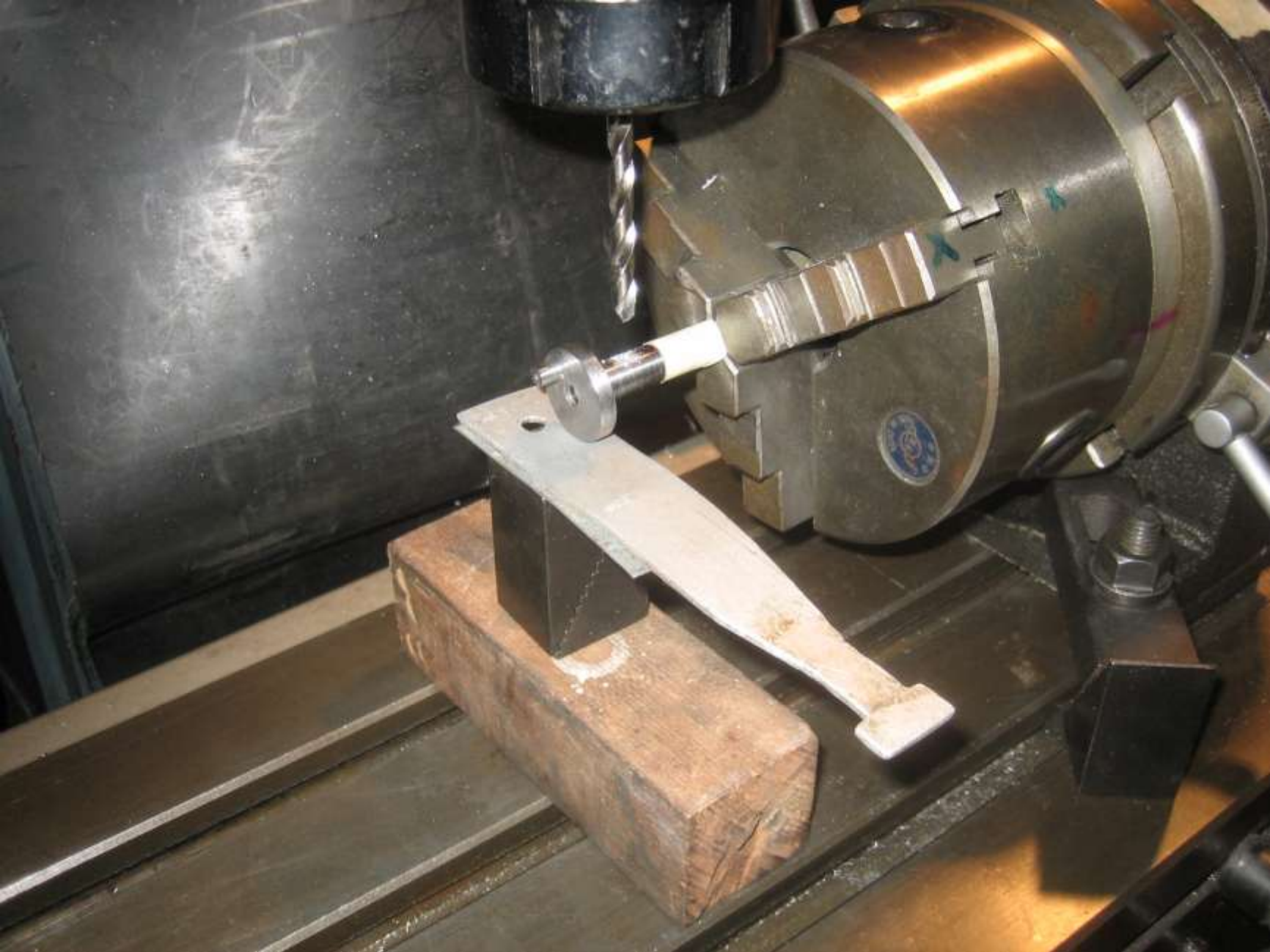
Drilling the hole to size – note support for the crankshaft end.
